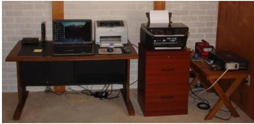
**Figure 7:** Home office (modem, router, laptop computer, black & white printer and color printer/scanner) powered by solar generator with module mounted on opposite side of back wall.
